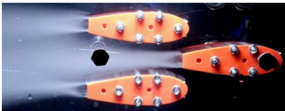
CIMYLEC profile in a hydrodynamic channel/tunnel
